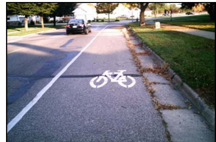
Example of a bike “sharrow” indicating a bike only lane
