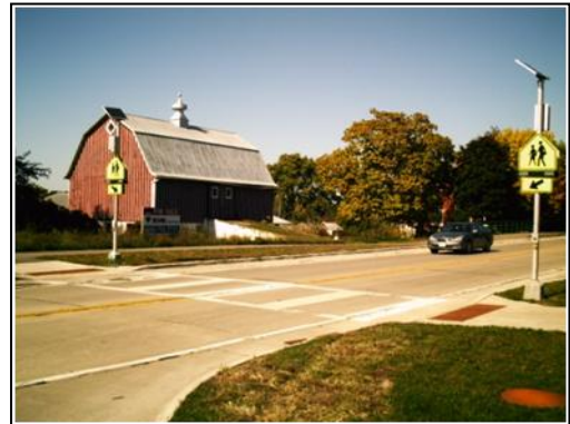
Example of a Rectangular Rapid-Flash Beacon crossing a possible solution for crossing State Highway 29
